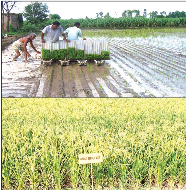
Demonstration of mat type nursery transplanting by self propelled rice transplanter
